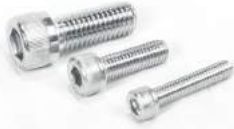
DIN 912 SOCKET HD CAP SCREW (ALLEN CAP SCREW) Grade: 304/316/202 Dai: M3-M16 Cold Forge Length: 6mm-120mm
