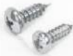
DIN 7981 PHILLIPS PAN HD SELF TAPPING SCREW Grade: 304/316 Dai: M2.9-M6.3 Cold Forge Length: 6.5mm-50mm
